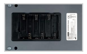
When batteries (type LR6) are used, 200 measurements with printing or 240 measurements without printing can be made with one set of batteries. The instrument displays a BAT icon on the LCD that gives information about the battery status.
