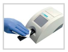
Figure 8: Cleaning the REF pad under the strip holder tray
