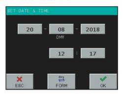
Pressing the OK button adopts the current time and date settings. The real-time clock in the DOASENSE Reader is powered by a built-in lithium battery. This battery is independent from the removable batteries.
